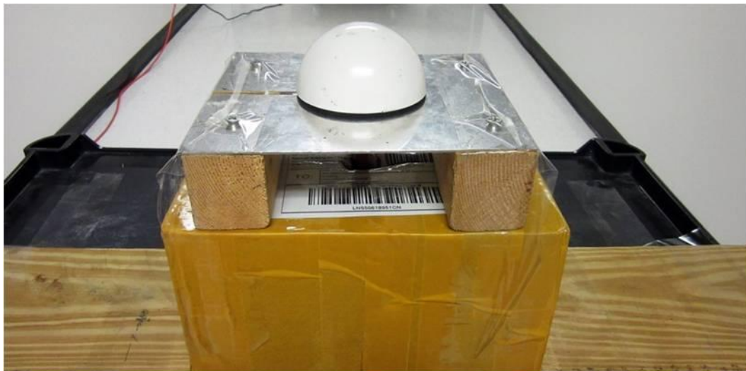
Figure 3.4 Mobile Mark DM2-5500 Receiver (Rx) Antenna, with extended ground plane, atop cardboard box and wooden board on cart.
