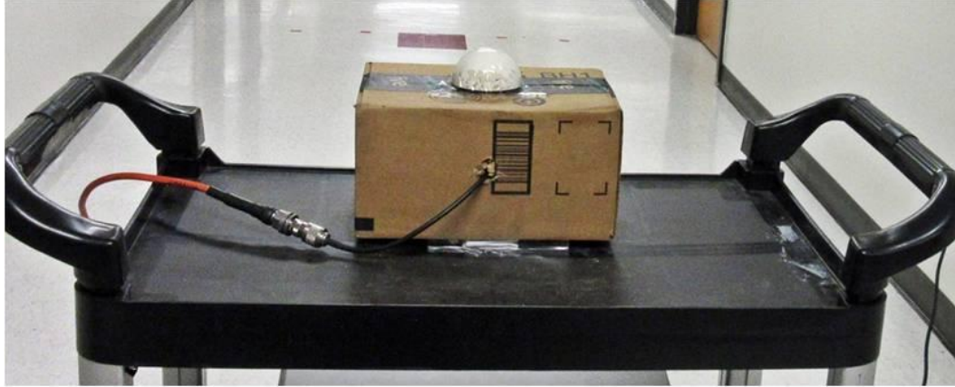
Figure 3.3 Mobile Mark DM2-5500 Transmitter (Tx) Antenna (within white radome) mounted in cardboard box atop equipment cart.
