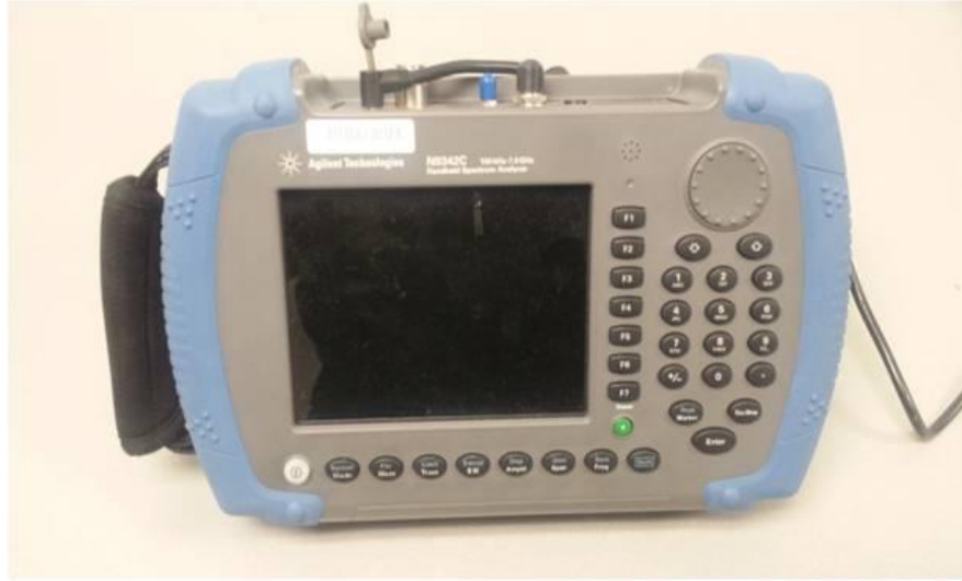
Figure 3.2 Agilent N9342C Spectrum Analyzer.
